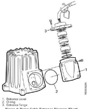
Figure 4: Pump Cable Entrance Diagram (Flygt)
